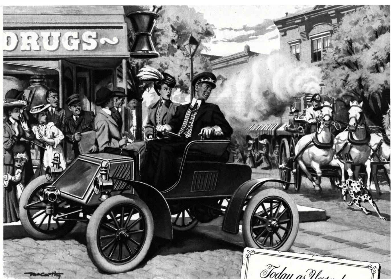
1902 RAMBLER was the first car offered by Nash Motors, then known as the Jeffery Company. This one-cylinder, twelve-horsepower model sold for \$750. 1500 were built in '02, one-sixth of all car production that year.
