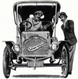
1908 COMPOUND was one of the few cars ever built with a three-cylinder engine. One of the three cylinders ran on the exhaust gases from the other two.
